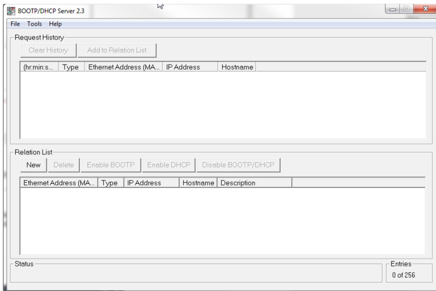
Figure 30: BOOTP/DHCP Server tool (Simple test tool from Rockwell) – BOOTP / DHCP server to assign IP addresses to devices on the network. Used for dynamic network configuration types (BOOTP, DHCP).
